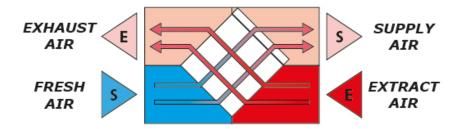
Supply and extract air flow in opposite directions through thermally conductive plates. As the warm extract air heats the plates, the cooler supply air absorbs this heat from the plates, achieving efficient heat exchange between the two air streams without them mixing. Heat transfer of 78% efficiency is attainable.
