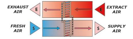
Run-around coils use the heat from the extracted air to preheat the supply air through a closed-loop heating coil system. While this method is less efficient in terms of heat recovery compared to other systems, it prevents any possible leakage between the incoming and outgoing air streams, making it ideal for settings where fully fresh air is critical, such as hospital operating theatres & where supply & extract units need to be remote from each other.
