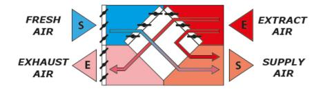
As an addition, the Plate Heat exchanger can be fitted with a recirculation damper arrangement, which allows a quantity of extract air to mix with the supply air. This configuration enhances energy efficiency by adjusting airflow as needed to maximize heat recovery, at early morning start up. This only works for applications where exhaust stream is suitable for mixing.
