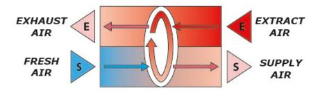
A slowly rotating wheel is constructed from thermally conductive materials, positioned between two air streams. One half of the wheel absorbs heat from the warm exhaust air, while the other half transfers that stored heat to the cooler incoming supply air.
